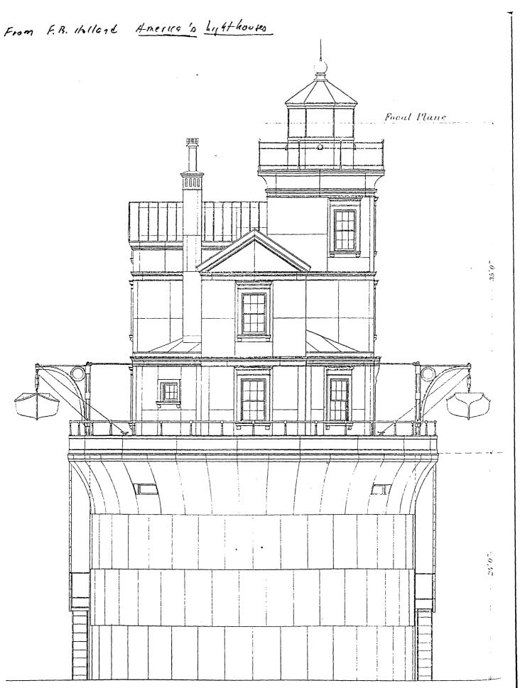
South and sectional elevations (1886) of the caisson lighthouse established in 1887 at Fourteen Foot Bank in Delaware Bay. The cast-iron caisson was floated into position and filled with concrete. Compare this elevation with the exterior photograph of Sandy Point (Maryland) light, on page 117. Drawing in the author's collection.
