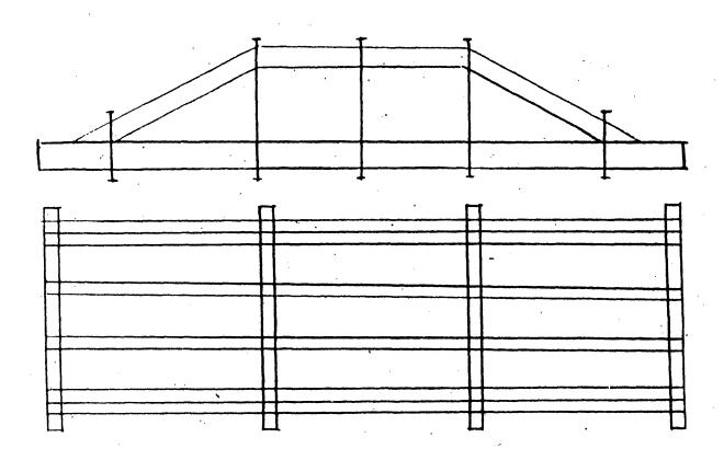
Figure 3. ORIGINAL FRAMING DIAGRAM FOR FARMINGTON CANAL BRIDGES
