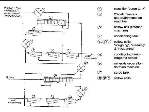
Fig. 2—Flotation Division, Timber Butte Mill (Gaudin 1932: 231)
