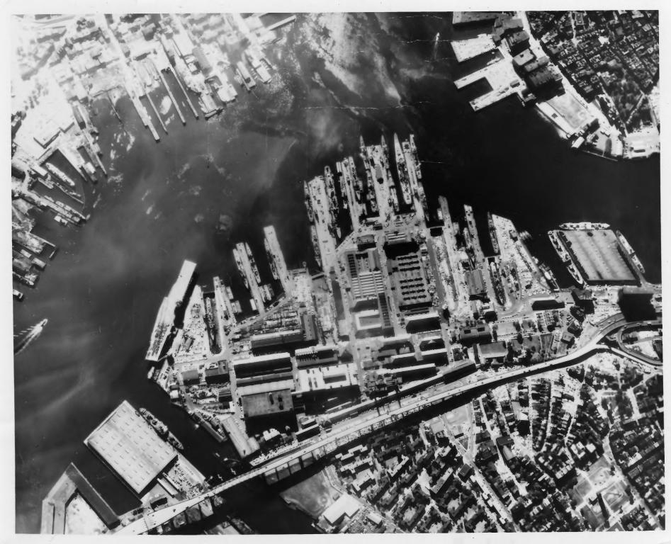
An aerial photograph of the Boston Naval Shipyard, Boston, Massachusetts. The yard lies above the elevated road. Dry Dock Number 1 is on the right in the picture and the ropewalk is the long structure that parallels the elevated road in the center of the picture.
