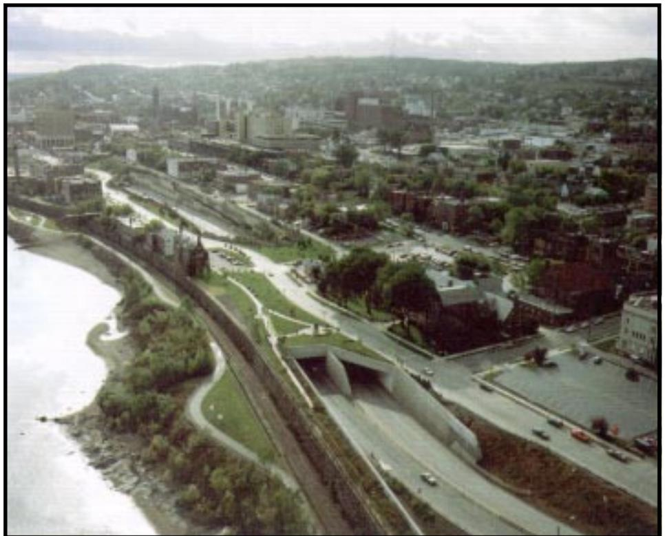
In many cases, there is a potential for designing a divided highway with independent horizontal and vertical alignments for each direction of traffic.
