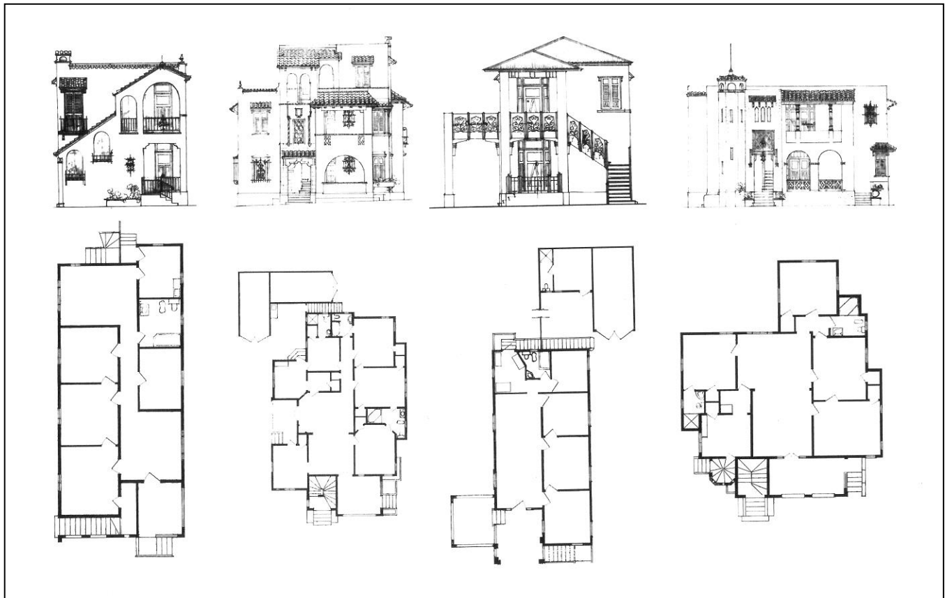
Figure 2. Examples of casa de apartamentos designed by Pedro de Castro (1895-1936), from left: Antonio J. Miró; Fernando Chardón; Arturo Bravo and; J. Abarca. The main elevations and their corresponding floor plans illustrate the interior layouts, but most importantly, the several locations, forms and relations between of the main staircase and service access.
