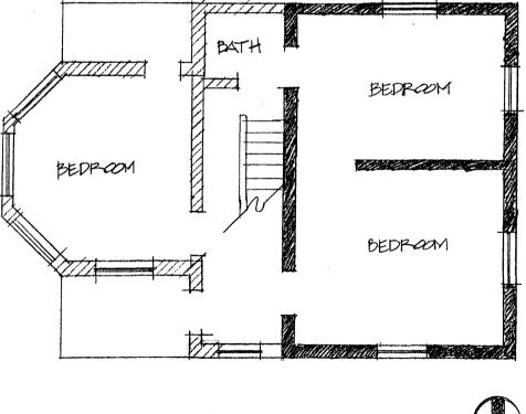
POLINS/ETRE HOUSE 113 W. MAIN, MINERSVILLE, UTAH SECOND FLOOR PLAN SCHEMATIC-NOT TO SCALE EZZZ C.1870
