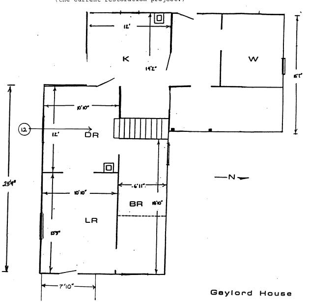
GAYLORD HOUSE FLOOR PLAN PRIOR TO WING REMOVAL (Wing reconstruction, based on this plan, is a goal of (the current restoration project.)
