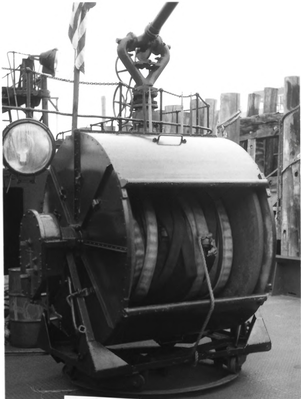
FIREBOAT FIRE FIGHTER NEW YORK, NEW YORK Owner: FIRE DEPARTMENT OF NEW YORK PROTECTED HOSE REEL MOUNTED ON BARBETTE AT FANTAIL.
