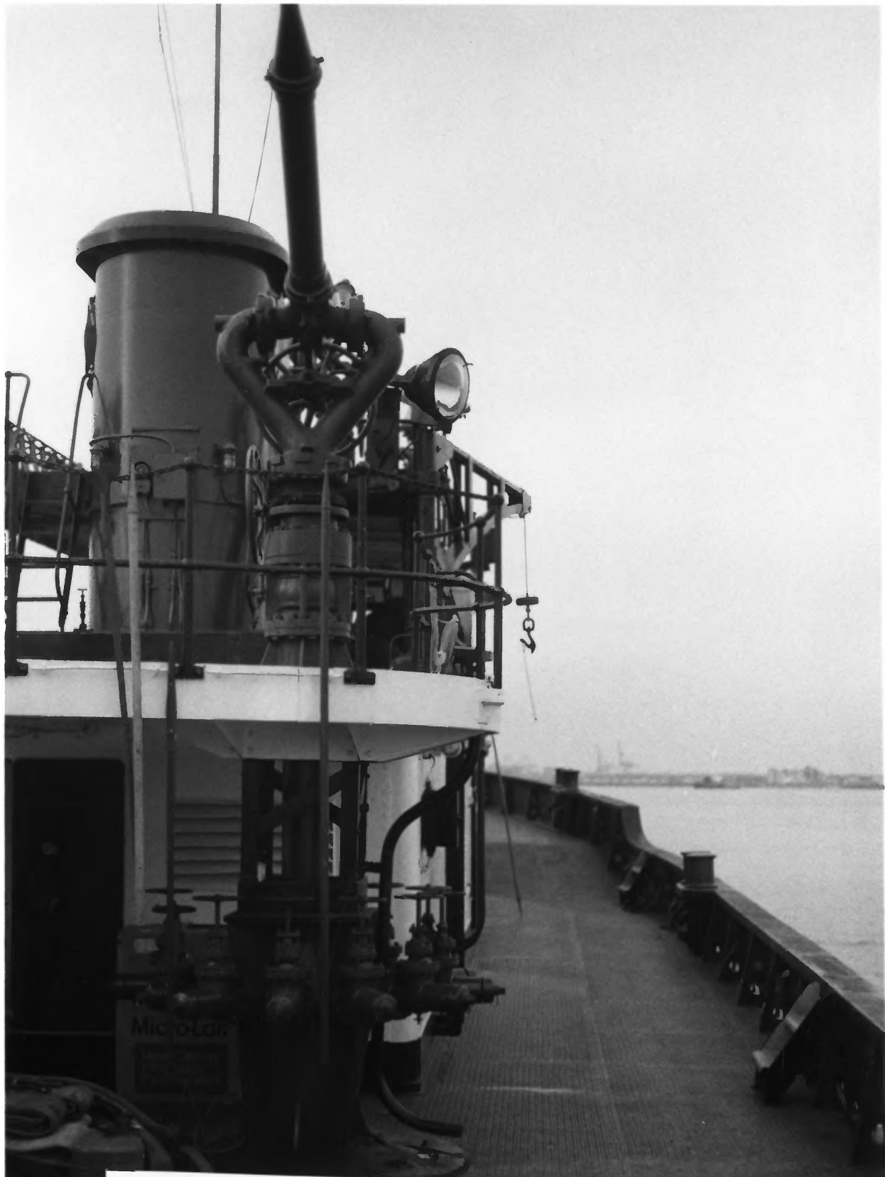
FIREBOAT FIRE FIGHTER NEW YORK, NEW YORK Owner: FIRE DEPARTMENT OF NEW YORK VIEW FORWARD, STARBOARD BEAM. NOTE THE MANIFOLD CONNECTION TO THE MONITOR. Photo #5 by JAMES P. DELGADO, 1988 Courtesy of: NATIONAL PARK SERVICE
