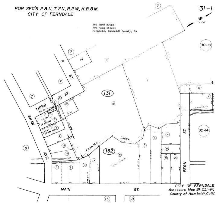
q FRANCES CREEK Α В S 6° 20'E 19.35' В С S 23° 52'W 60.15' С D S 2° 56'E 47.45 D S 48° 20'W 58.45' Ε Ε S 18°9'E 32.05' F F G S 51° 37'E 2.60' G н S 51° 37'E 46.35' ΗI S 5° 44'E 57.05' Ι J \$ 36°44'W 71.10' κ \$60° 40' W 59.70' J ĸ L S9°26'E 89.55' S13° 35'E 76.40' М L М ٨ S 3º 52'W 61.05'
