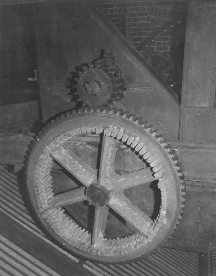
Huge bull-wheel with wooden teeth and wedges located in corrugated sheet metal roof over silos. West brick wall and one of many rope-driven wheels are in background.
