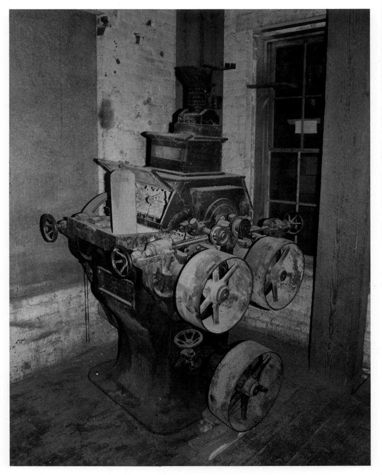
Late 1800's Allis-Chalmers belt-driven milling machine located on first floor.
