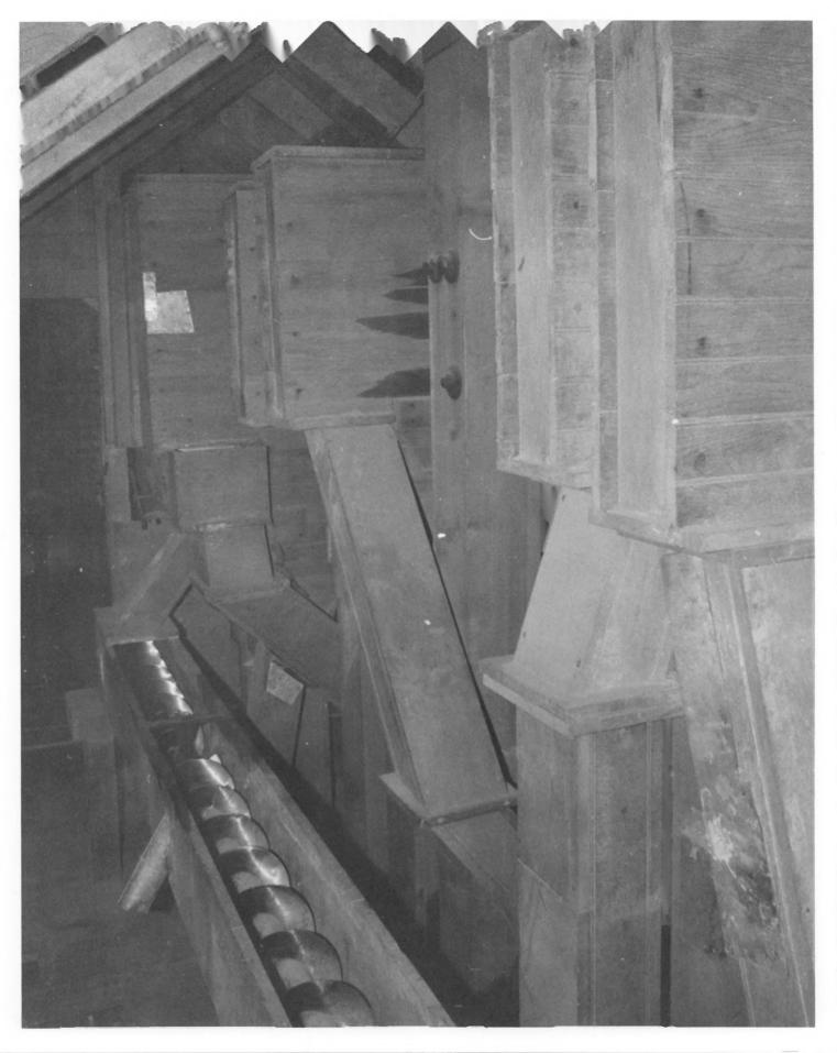
Screw conveyor and chutes in loft area over third floor (looking in direction of silos to the west).
