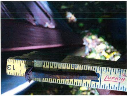
Photo 7 - Typical siding nail, removed (and replaced) without the use of tools.
