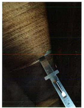
Photo 28 - Penetration into visible urethane foam=3/4"
