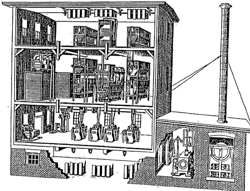
Fig. 8 Cutaway view of an 1892-roller system flour mill. This represents one of the Edward P. Allis Co.'s latest fifty-barrel flouring mill, the building being 30x40 ft., with basement and three stories. The mill house is of frame and the engine room is of brick. Note the increased height of the second story. (From their catalogue "Small Modern Mills" as reprinted in *United States Miller*, (Dec. 1892), 271).
