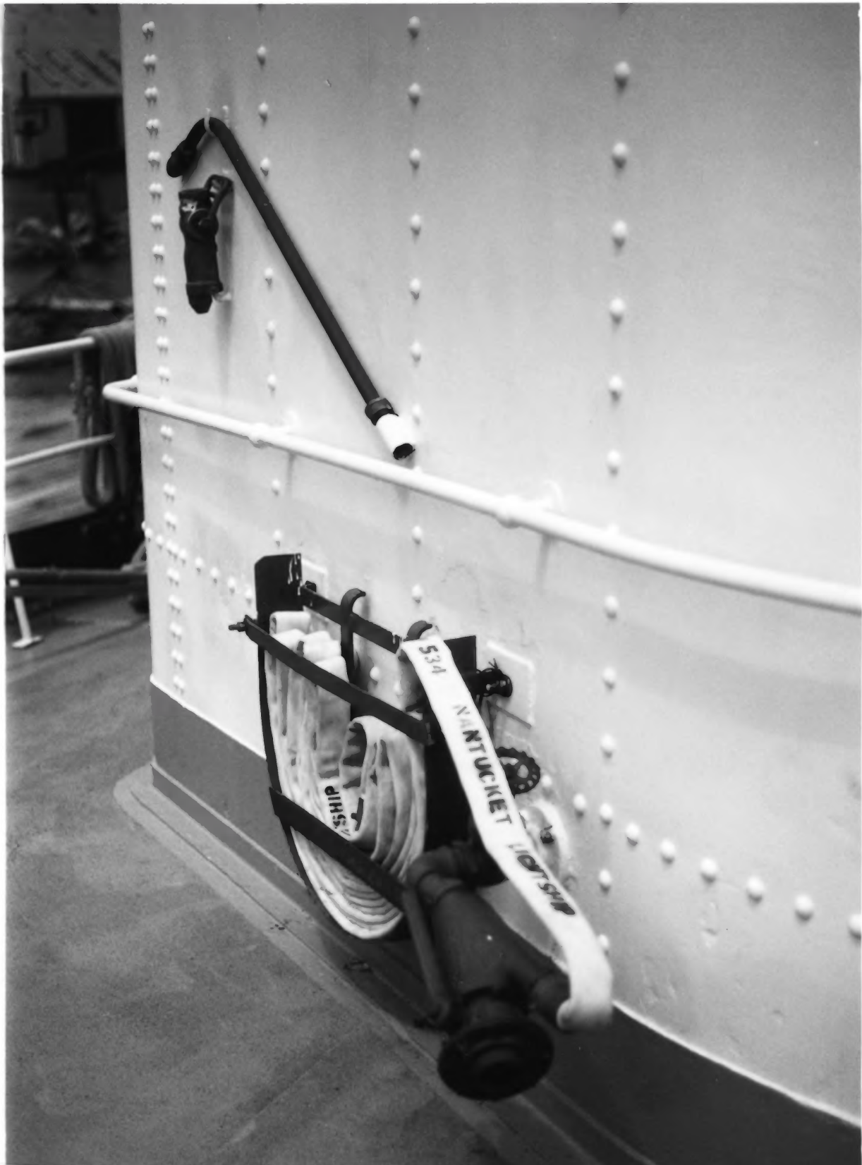
LIGHTSHIP NO. 112, NANTUCKET SOUTH PORTLAND, MAINE Owner: NANTUCKET LIGHTSHIP PRESERVATION FIREFIGHTING GEAR AND HOSE ON THE PILOT- HOUSE. NOTE THE STENCILLED FIRE HOSE. Photo #6 by JAMES P. DELGADO, 1989 Courtesy of: NATIONAL PARK SERVICE
