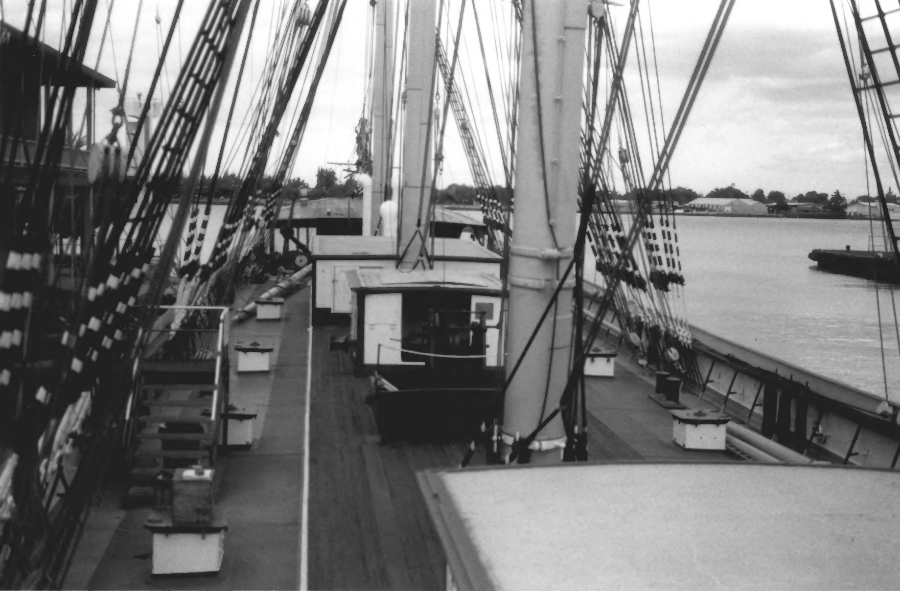
FALLS OF CLYDE , Honolulu, Hawaii National Park Service Photograph by James P. Delgado, 1988 Hawaii Maritime Center, Inc. Deck view showing deckhouses, forecastle, wooden and steel sections of the weather deck and oil tank expansion trunks. Photo #5
