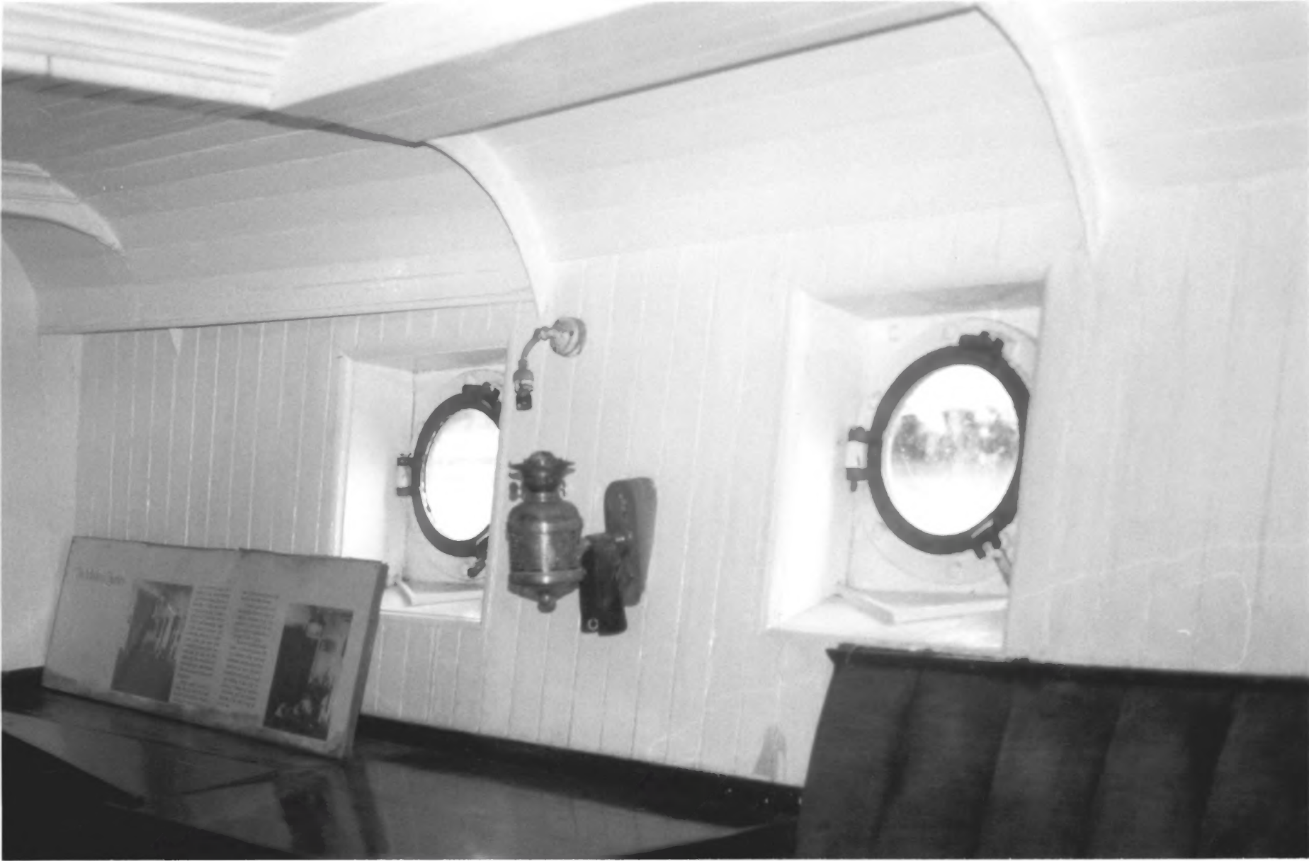
FALLS OF CLYDE , Honolulu, Hawaii National Park Service Photograph by James P. Delgado, 1988 Hawaii Maritime Center, Inc. Typical joiner's work--master's stateroom. Note deadlights. Photo #9
