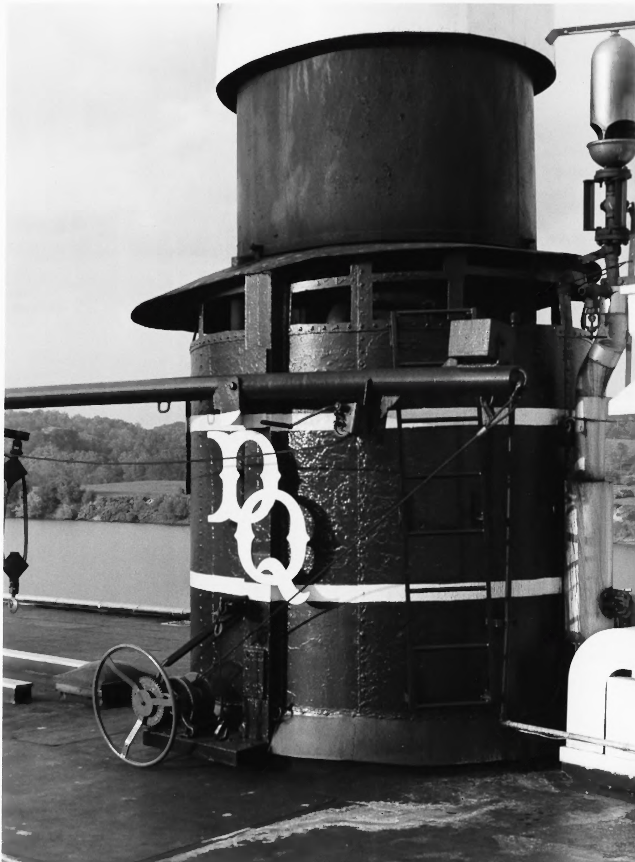
DELTA QUEEN NEW ORLEANS, LOUISIANA Owner: DELTA QUEEN STEAMBOAT COMPANY TELESCOPING SMOKESTACK Photo #5 by KEVIN J. FOSTER, OCTOBER 9, 1988 Courtesy of: NATIONAL PARK SERVICE
