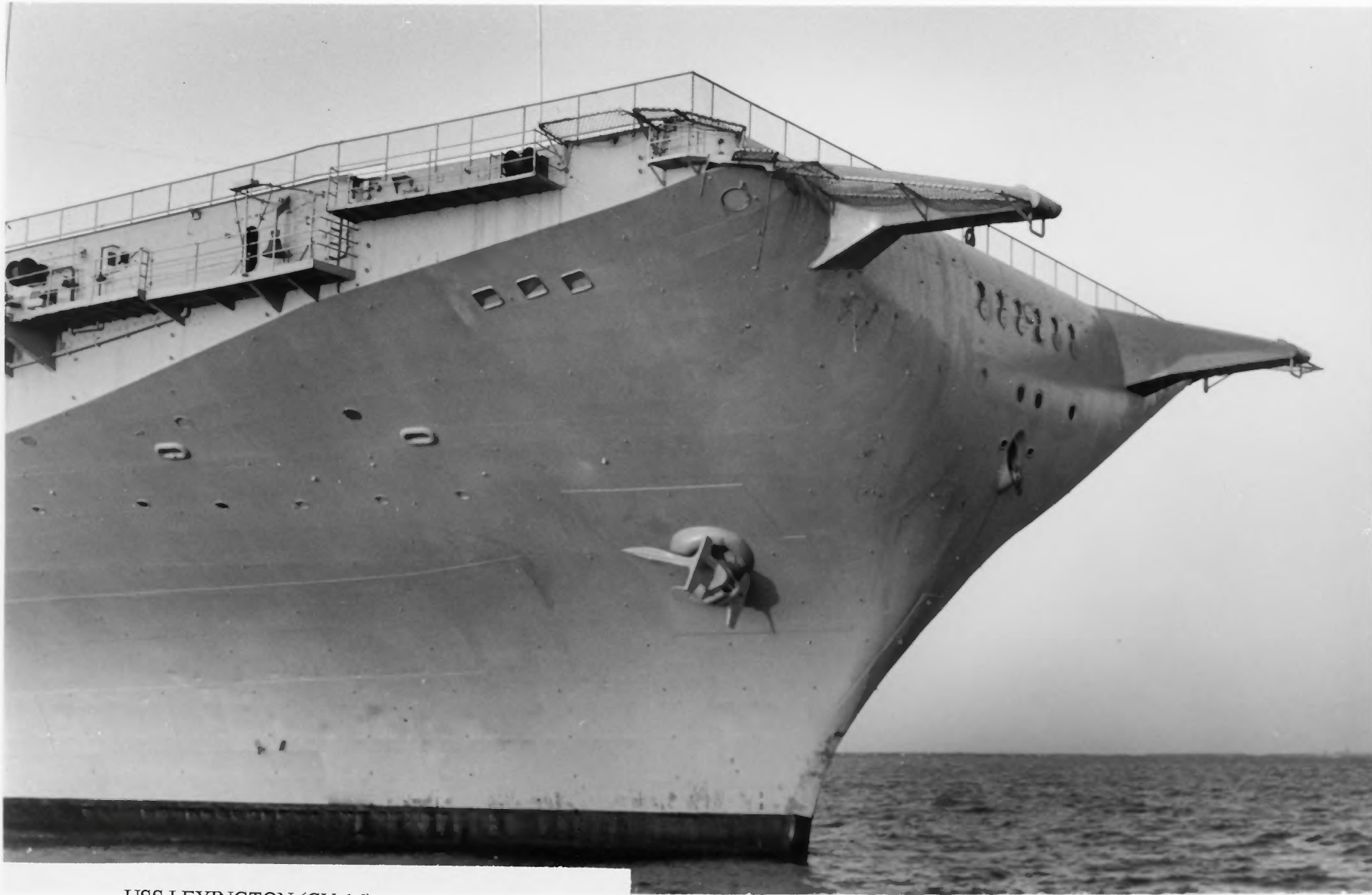
USS LEXINGTON (CV-16) Corpus Christi, Texas The ship's "hurricane bow," 1996. Photographer: Hugh Power
