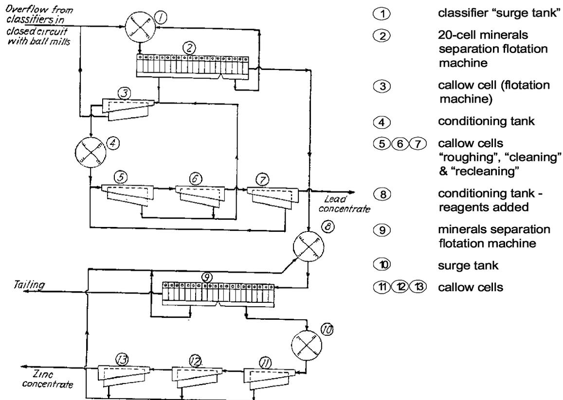
Fig. 2—Flotation Division, Timber Butte Mill (Gaudin 1932: 231)
