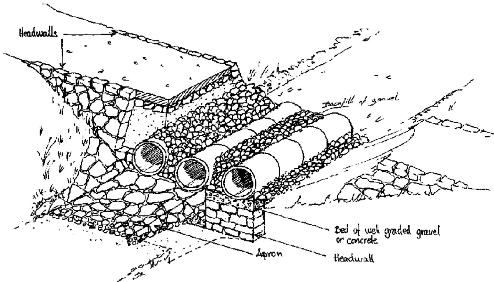
Accompanying Documentation - Culvert Construction using Pipes
