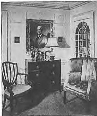
Not only the walls and ceilings in this house are pressed wood, but even the family portraits have been painted on it. Solid wood is used for doors and cabinets since pressed wood is made in sheets not much thicker than 1/4"
