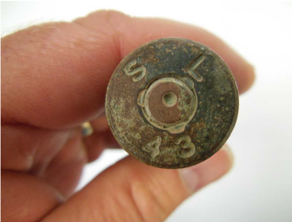
.50 Caliber Casing Showing Manufacturing Location and Date Stamp on Bottom
