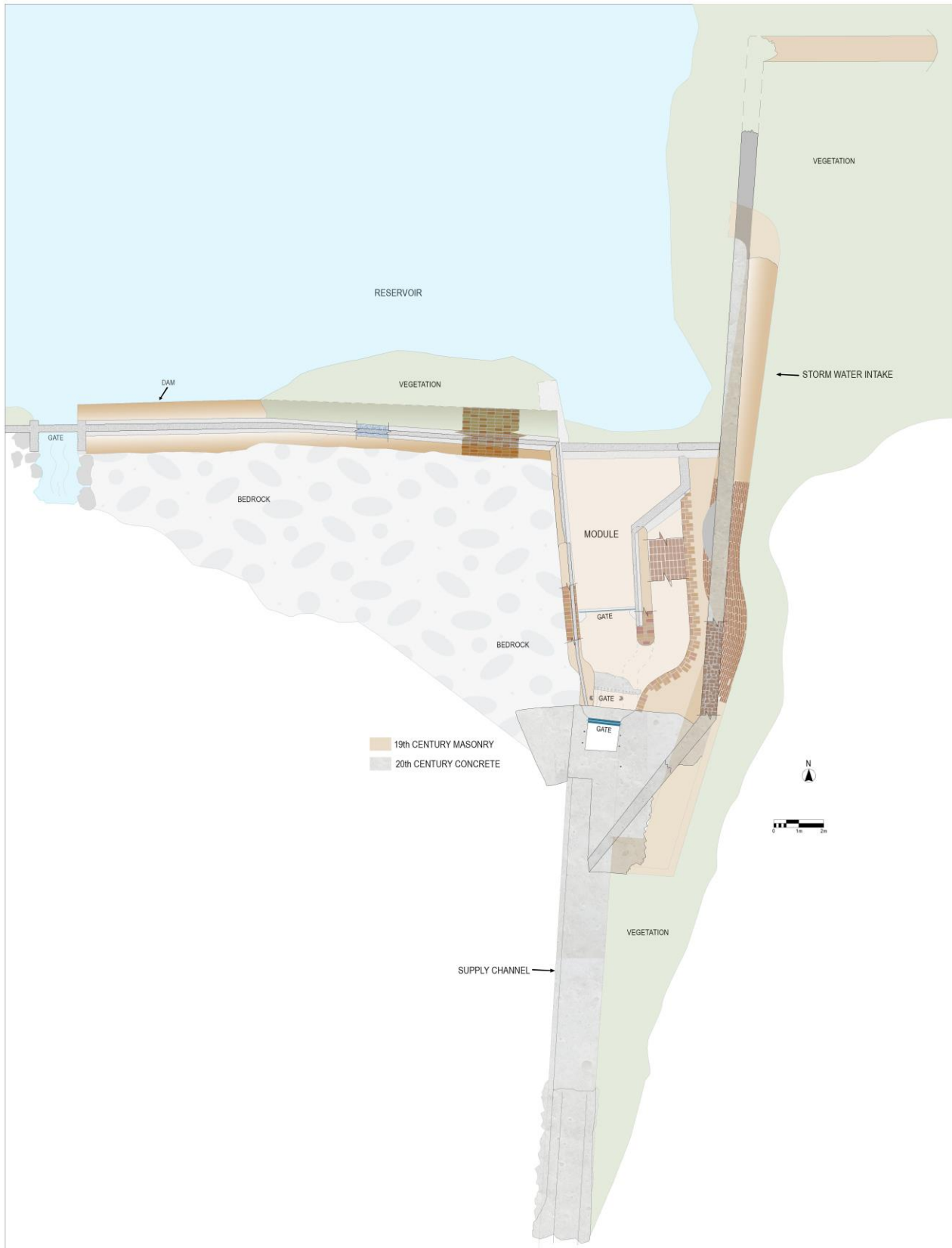
Drawing of the dam and modules of the Tres Haciendas Irrigation System
