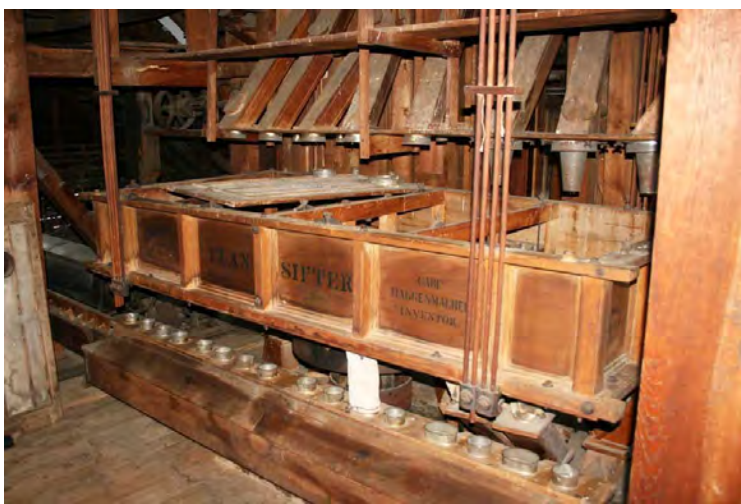
Figure 6. Bernard & Leas plansifter (Carl Haggemacher, Inventor) in current use (2016) at Thorp Mill, Thorp, Washington. "Thorp Mill," accessed July 17, 2016, http://www.thorp.org/grist-mill-diagram/
