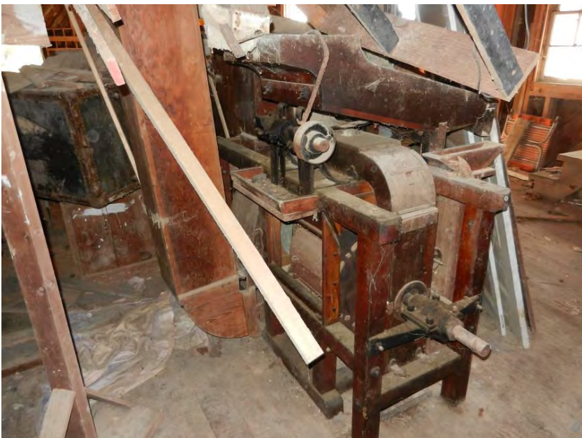
Photo 16: WV_JeffersonCounty_Feagans'Mill_016 Feagans' Mill, First Floor, Facing South, Sifter
