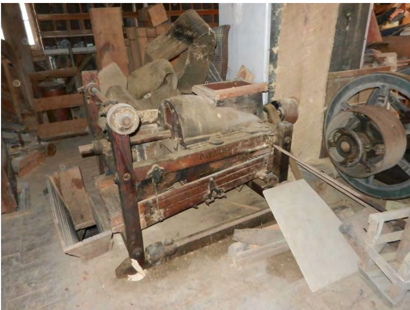
Photo 14: WV_JeffersonCounty_Feagans'Mill_014 Feagans' Mill, First Floor, Facing East, Union Ironworks Corn Grinder
