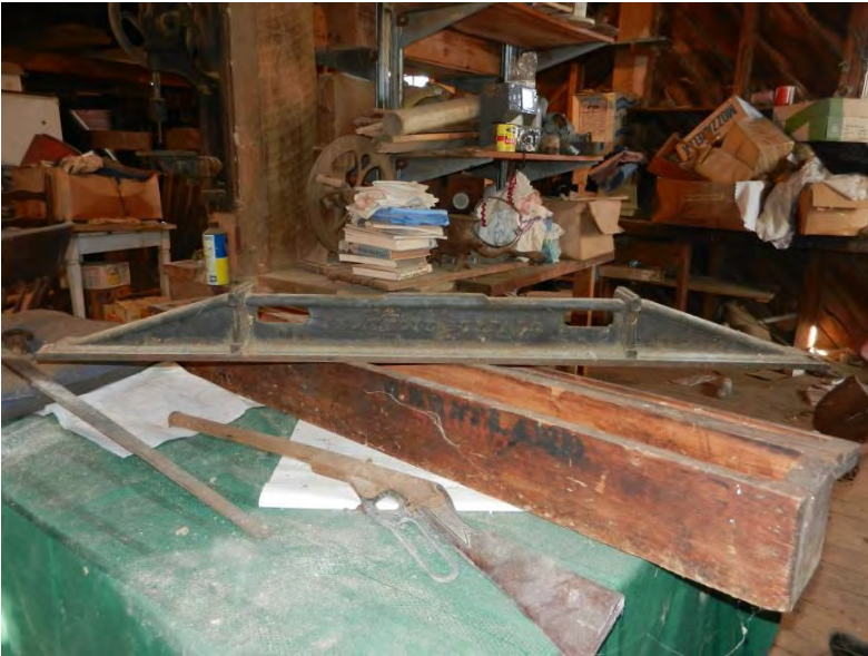
Photo 27: WV_JeffersonCounty_Feagans'Mill_027 Feagans' Mill, Second Floor, Buhr Stone Leveler made by "Jno. T. Noye Buffalo"
