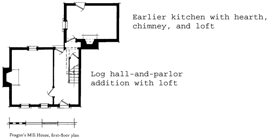
Figure 3. Architectural Rendering. Floor plan of Feagans' Miller House circa 1820. In John C. Allen, Uncommon Vernacular: Early Houses of Jefferson County, West Virginia, 1735 – 1835 . Morgantown: West Virginia University Press, 2011, 72. Rendering by Andrew Lewis. Allen posits that a builder attached a log hall-and-parlor structure to an older kitchen.
