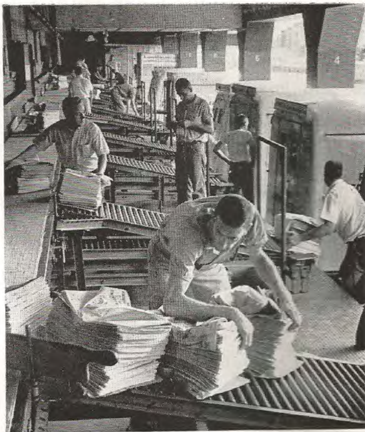
Bundles slide down circular chutes to loading dock where they move on endless belts to proper truck.
