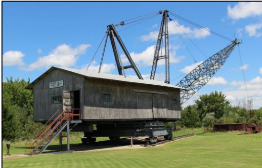
Page Dragline Model 222 (1920) - 46' L x 28' W (cab) - 100' boom - 3 cu. yd. bucket
