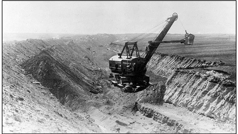
Figure 26: Bucyrus-Erie 320-B, showing how it worked within the landscape (Univ. of Saskatchewan)
