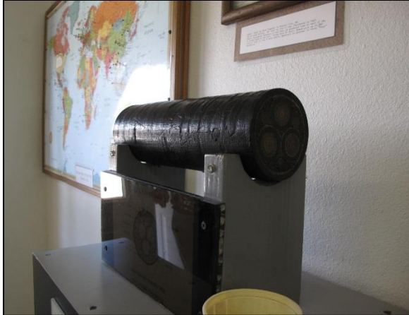
Figure 14: Sample of the power cable
