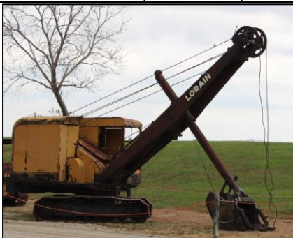
Lorain Tracked Excavator (ca. 1954) - 20' H x 28' L x 9'-9" W - 3/4 cu. yd. bucket
