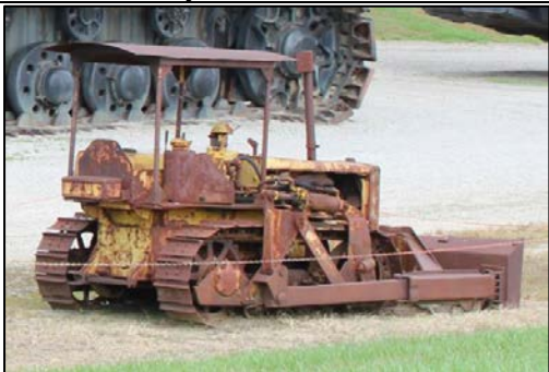
Caterpillar D4 Bulldozer (1947) - 7'-7" H (top of cab) x 12'-10" L - 8'-0" W (with blade)
