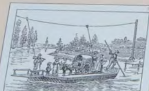
A typical ferry on a small river was held in place by a cable and pushed across the stream with a pole.
