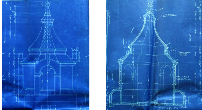
Figure 3 and Figure 4. Elevation and section of Building A tower, 1925-1928, Joseph O’Kelly, Instituto Loaiza Cordero para Niños Ciegos Historic District. 5
