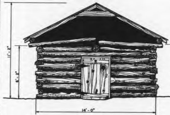
○ NORTH ELEVATION SCALE: 1/2" = 1'-0"
