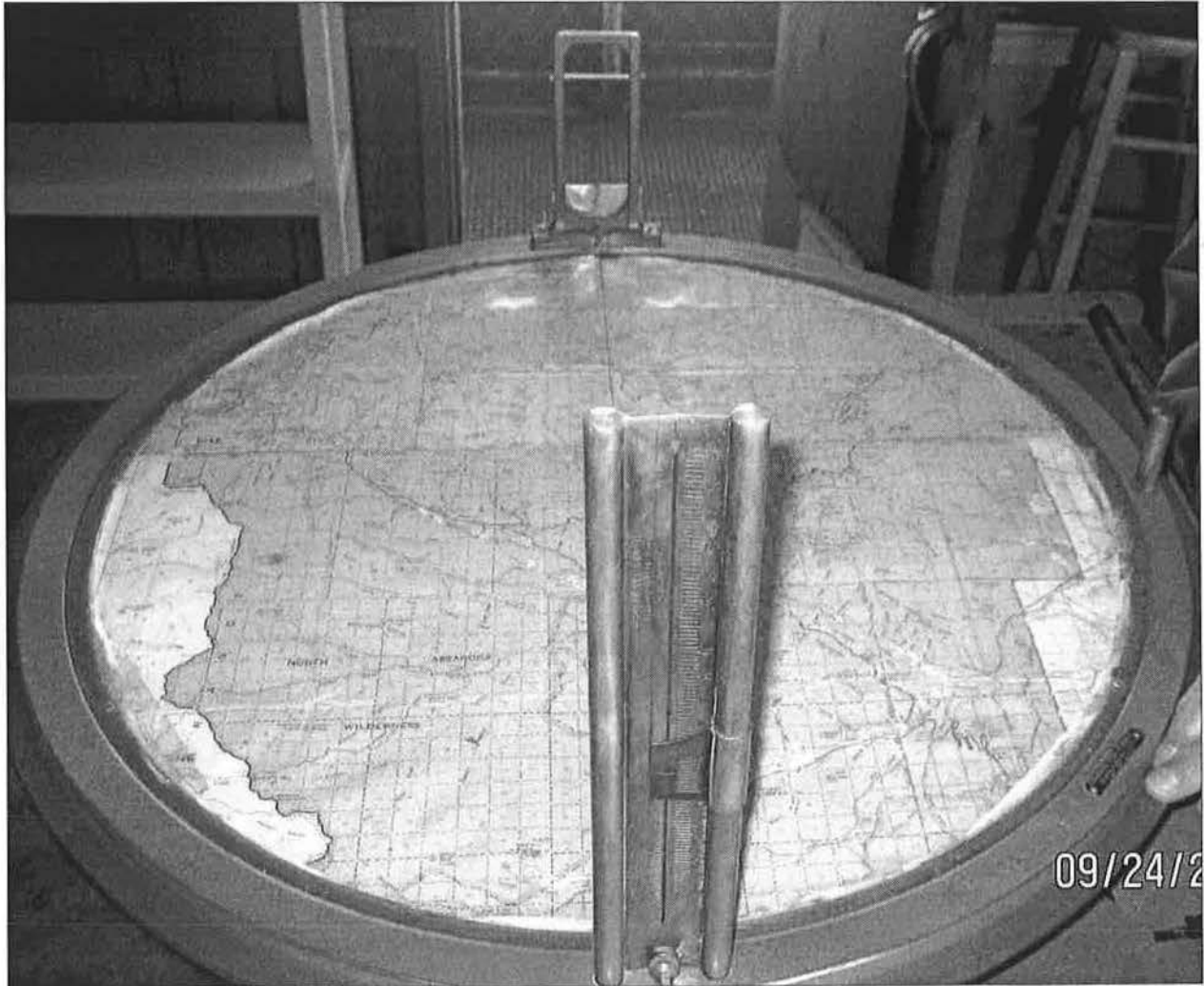
Figure 15. Osborne Firefinder, used to pinpoint the location of forest fires, 2009 (courtesy Friends of Clay Butte Tower)
