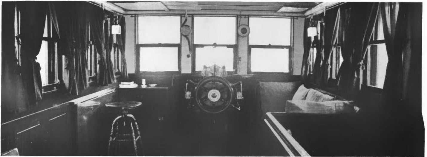
The boat is handled from the deckhouse, which is placed well forward.
