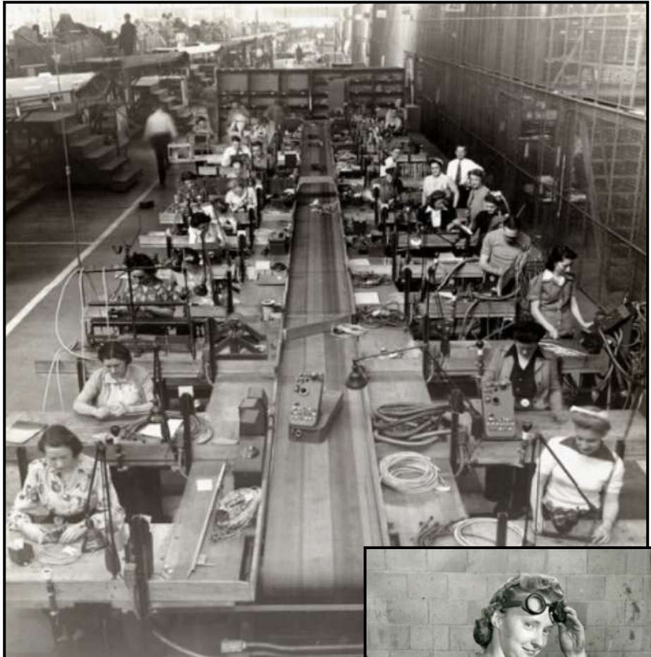
Figure 29: Top, women doing electrical sub-assembly work at Curtiss-Wright; bottom, woman grinding machined part; both 12 March 1943. Source: Missouri Historical Society, F. Dale Smith Collection, ID# N30461 (top); ID# N34371 (bottom).
