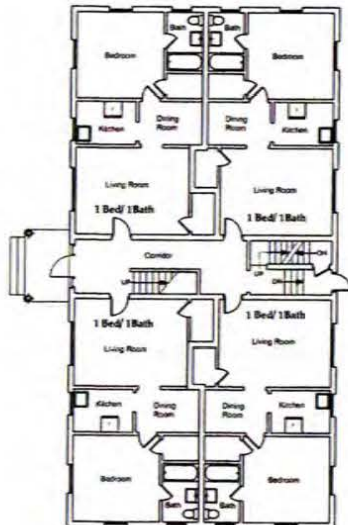
5 BUILDING C FIRST FLOOR PLAN SCALE 1/8" = 1'-0"
