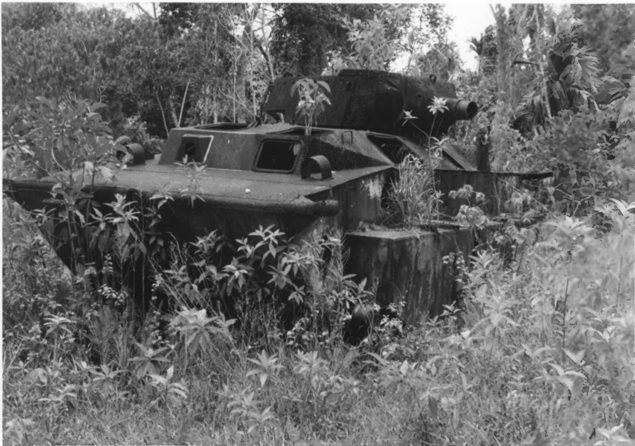
6. Peleliu. American landing craft, LVT(A)4, with a turret mounting a 75mm howitzer. It stopped near the southern base of the Umurbrogol Mountain complex.
