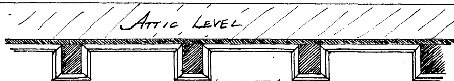
A. SKETCH ILLUSTRATING THE MANNER IN WHICH SIMPLE CROWN MOULDING IS MITERED AROUND EXPOSED BEAMS WHERE THEY MEET THE WALL, IN SECOND FLOOR ROOMS.
