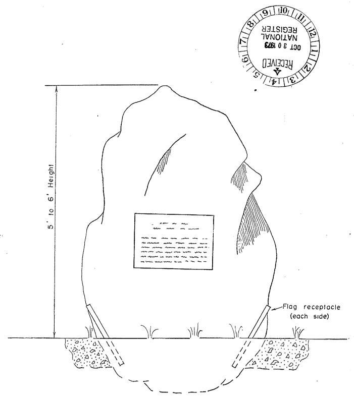
Place 6" of reinforced concrete around base of boulder to minimize possible settlement.
