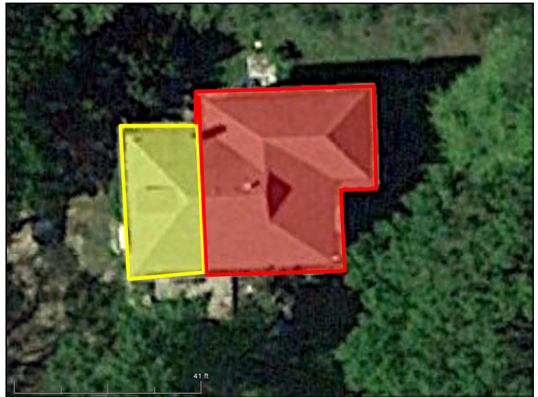
Figure 2: 2014 Aerial image of house, showing original block of house (left) and 1870s block (right). A second story was added to the left portion in 1922. North is up.
