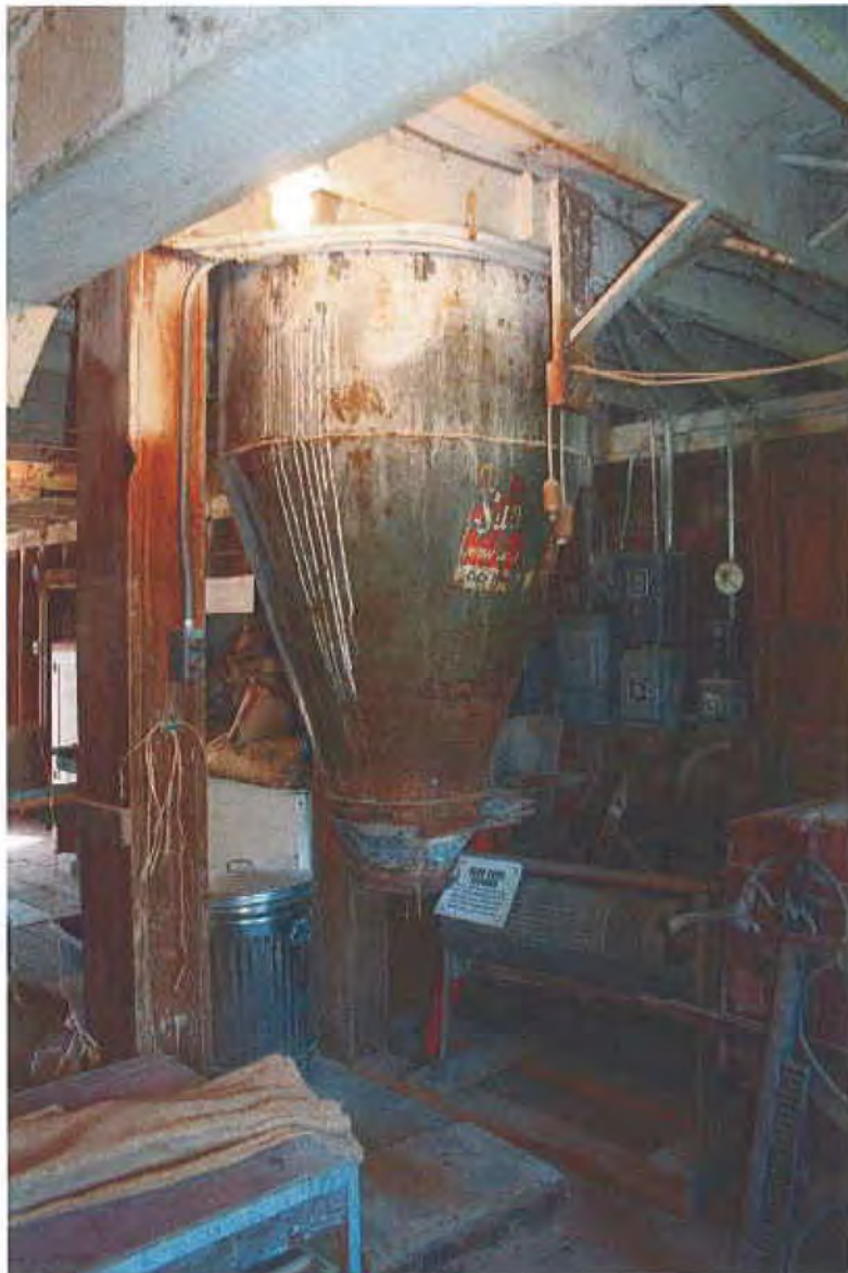
Photo 11. Interior view – First floor – Chicken Feed Mixer (F)
