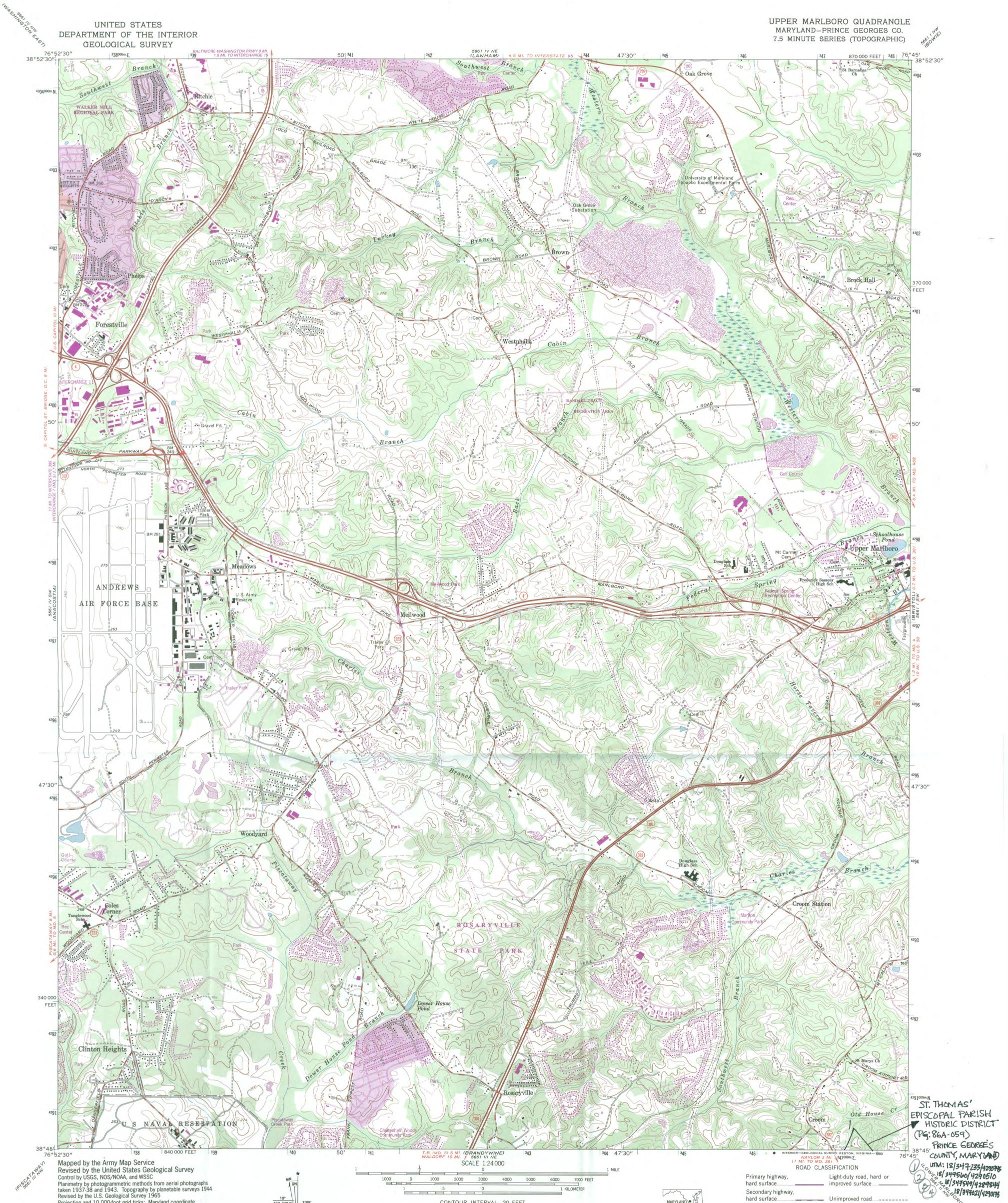
Projection and 10,000-foot grid ticks: Maryland coordinate system, (Lambert conformal conic) 1000-meter Universal Transverse Mercator grid ticks, zone 18, shown in blue 1927 North American Datum (NAD 27)
