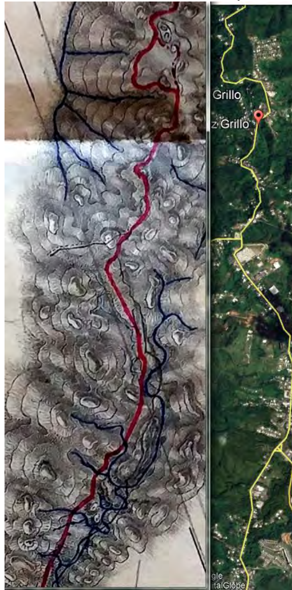
Figure 27. The image presents an overlapping of Bayo's 1875 drawing with the propose route from Caguas to Cayey, and a 2018 Goggle's map view with today Carretera Central 's footprint.
