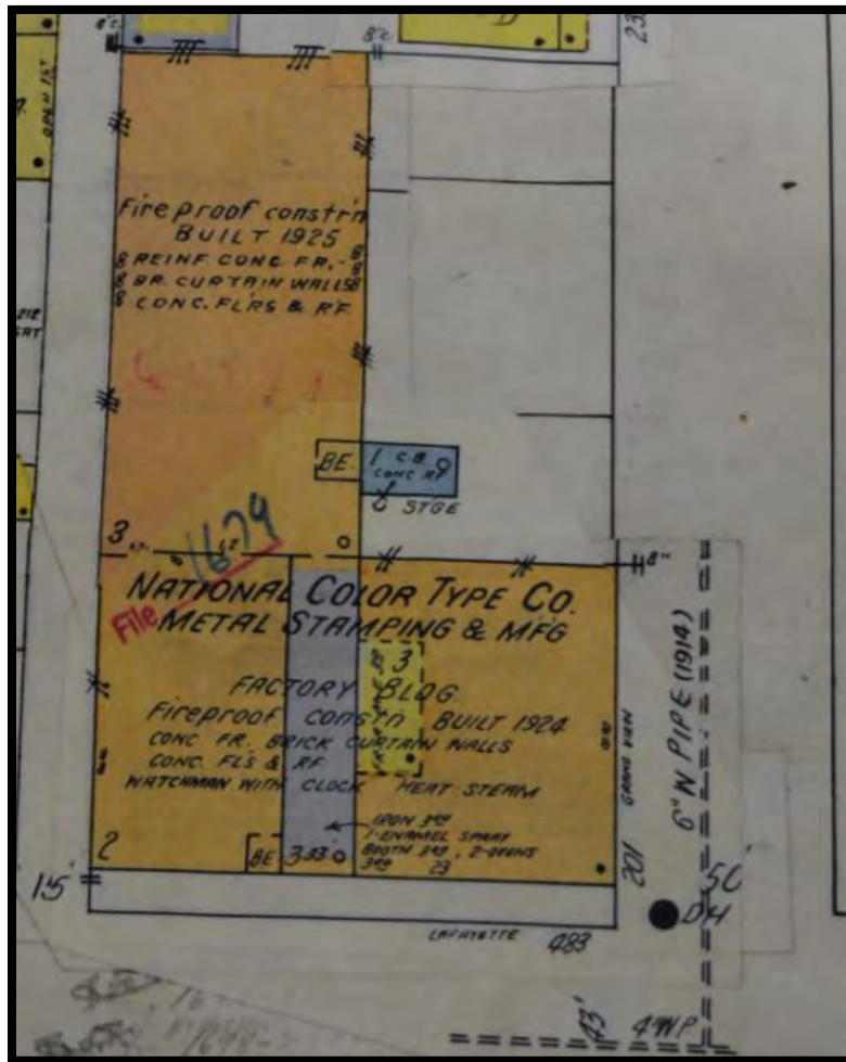
Figure 3. 1910 Sanborn Fire Insurance Map, revised to August 1941. Note that the circa 1946 one-story addition (C) was not in place at this time and that the 1924 portion of the building (A) was only two stories tall and the 1925 addition (B) was three stories in height. Also, the 1925 addition was missing its last four bays with elevator and stair shaft, which was appended to the rear of this portion of the building circa 1946. 4
