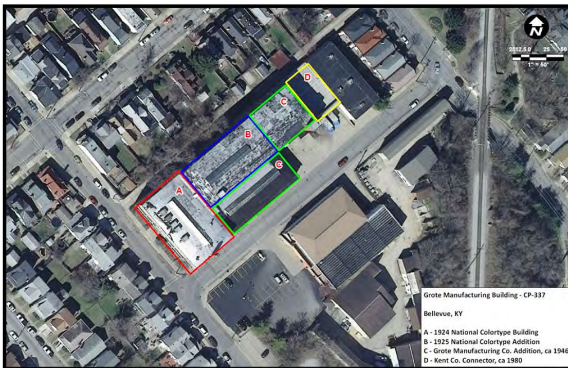
Figure 2. National Colortype/Grote Building graphic showing additions in aerial view. Note that the Kent Company Commercial building directly east shares a party wall with the main factory building (A-D), but is not associated with this building during its period of significance.
