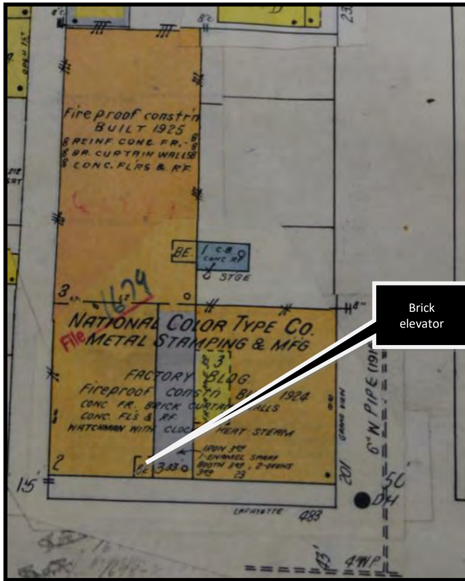
Figure 24. Grote Building Sanborn Fire Insurance map view, August 1941. BE notes brick enclosed elevator with wire-glass doors. Note that the circa 1946 addition had not yet been constructed.
