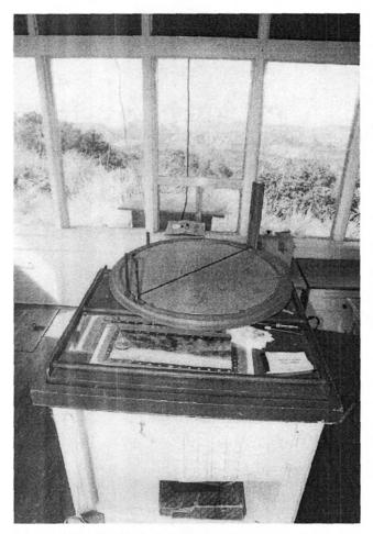
Figure 109. The Osborne Firefinder was installed in the Lookout shortly after construction.
