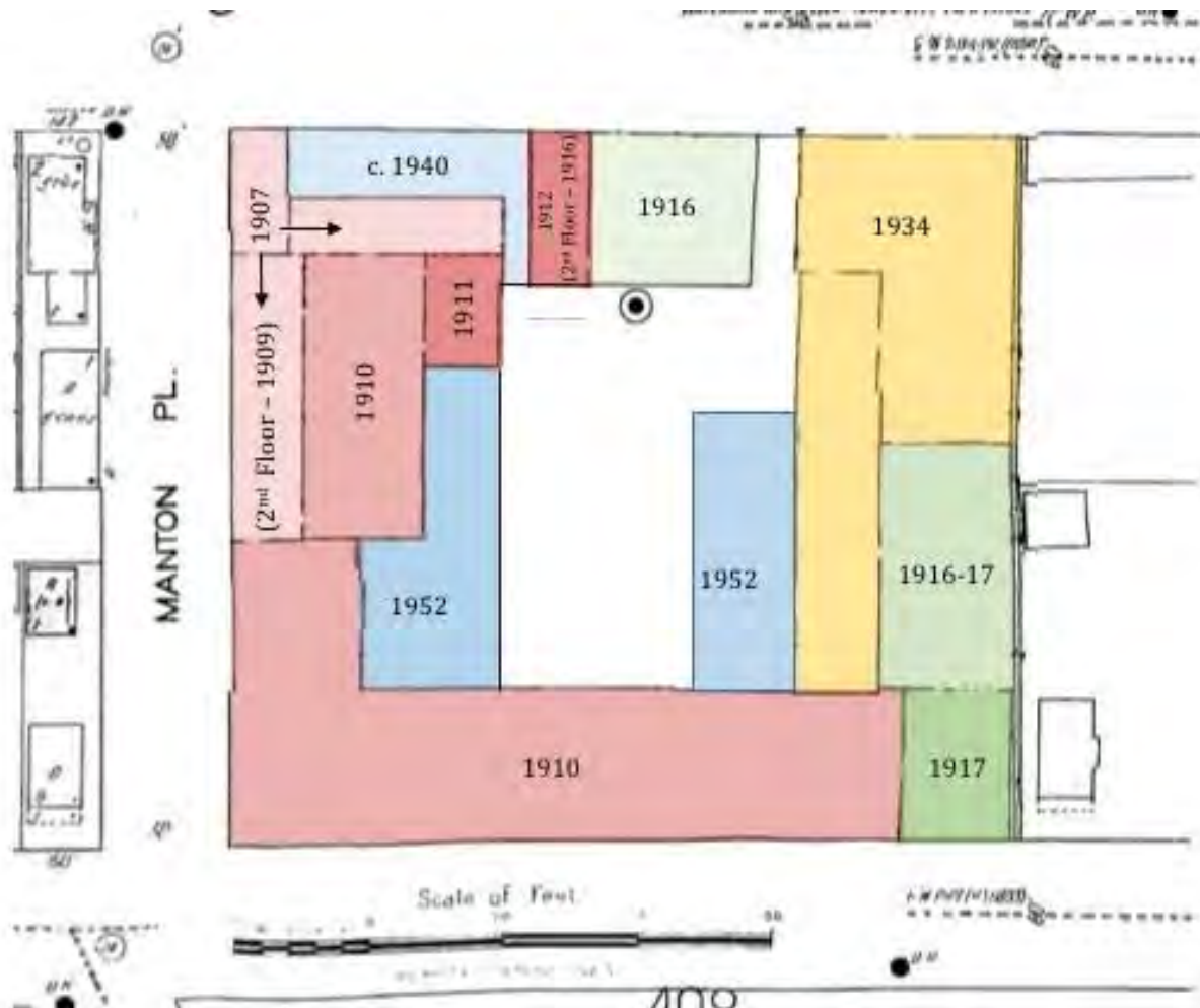
Diagram showing the dates of construction for each addition to the facility.
