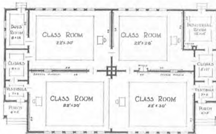
FLOOR PLAN NO 400 FOUR TEACHER COMMUNITY SCHOOL TO FACE EAST OR WEST ONLY
