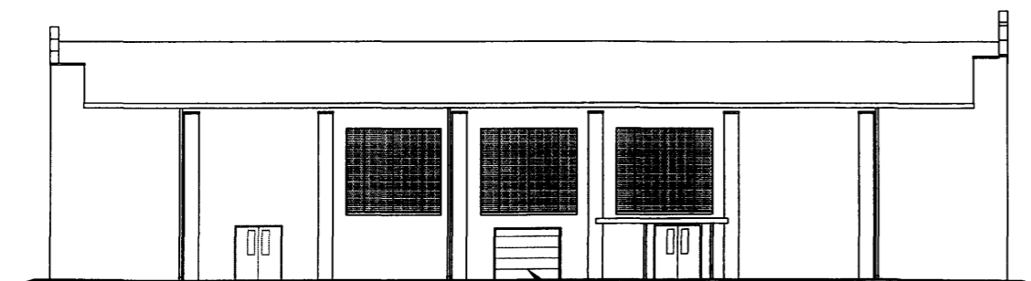
BUILDING ELEVATION SOUTH FACE 2 A2.5 Scale: 3/32" = 1'-0"
