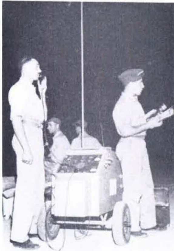
Figure 14. Using a portable transmitter and receiver to control flight traffic during night training at Falcon Field. Reproduced from A.L. Storrs, "Falcon Offers Night Flying Suggestions," The Thunderbird , Vol. 1, No. 4, June 1943, 2.
