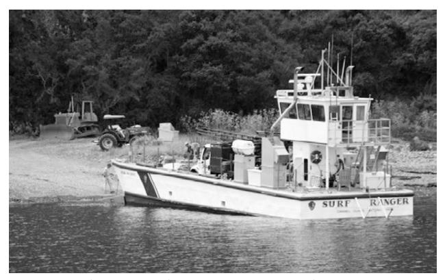
Figure 5-13. The *Surf Ranger* landing craft is used to move large items to and from the islands including trash removal trucks, building supplies, and vehicles.
