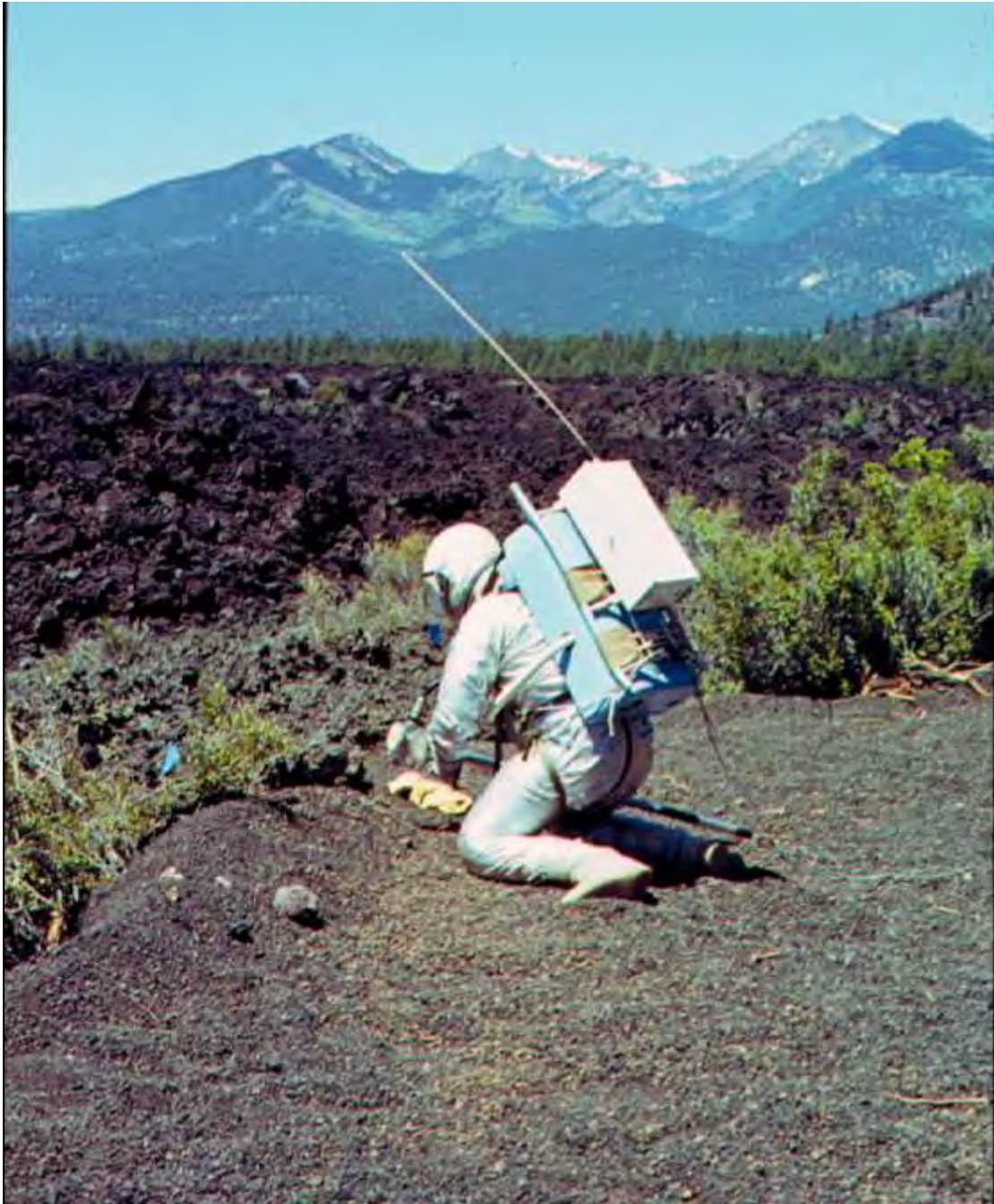
Fig. 10. Suited test subject collecting a sample on the northern edge of the Bonita Lava Flow. Note the mock Personal Life Support System. (Image from Schaber, open-file report, 2005).
