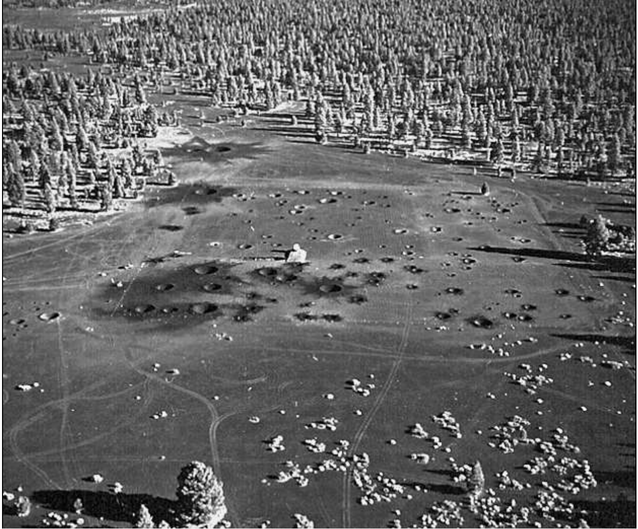
Fig. 19. The final appearance of Crater Field One after the addition of 96 craters in October, 1967. In total, the field contains 143 craters of varying size. Note the ramp at the center of the field that was used to simulate the height of the lunar module on the moon. A fence surrounding the field is also visible. (Image from Schaber, open-file report, 2005.)
