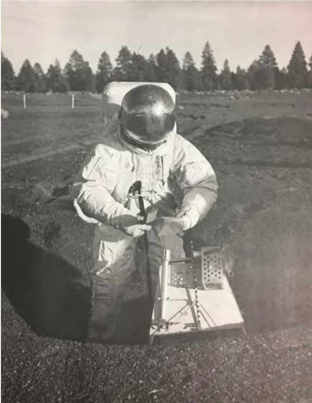
Fig. 73. Suited test subject with lunar hand tool carrier. (Uncatalogued USGS Image, USGS Astrogeology Regional Planetary Information Facility, USGS Astrogeology Science Center, Flagstaff, Arizona.)
