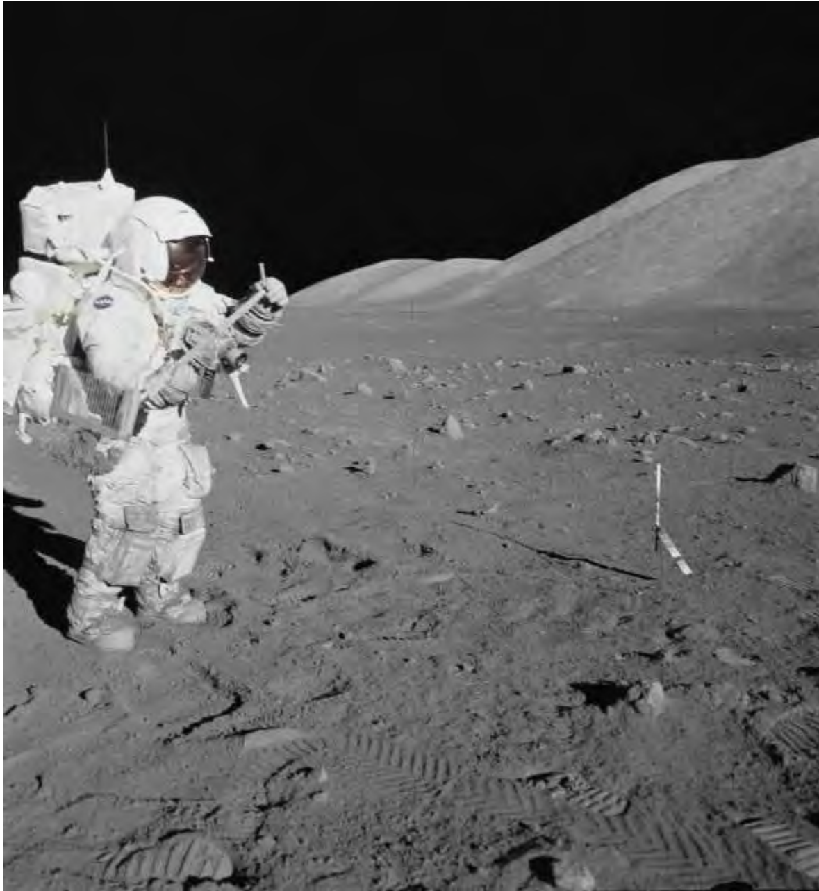
Fig. 66. Astronaut Harrison H. Schmitt holds a lunar rake used for sampling small rocks during an EVA for Apollo 17. Schmitt and other astronauts practiced sampling with these tools in the district. (December 11, 1972. NASA photo AS17-134-20426.) Image available from: https://spaceflight.nasa.gov/gallery/images/apollo/apollo17/html/as17-134-20426.html
