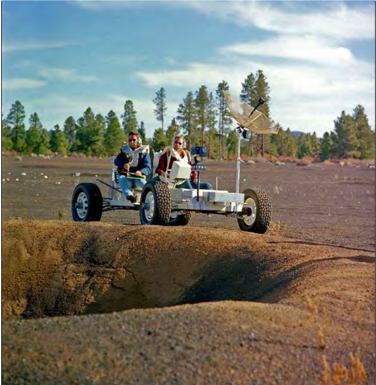
Fig. 61. Apollo 15 astronauts Jim Irwin (left) and Dave Scott (right) train in the USGS LRV simulator Grover on one of the Cinder Lake crater fields, 1970. (Image from Schaber, open-file report, 2005. NASA photo AP15-S70-53283.)
