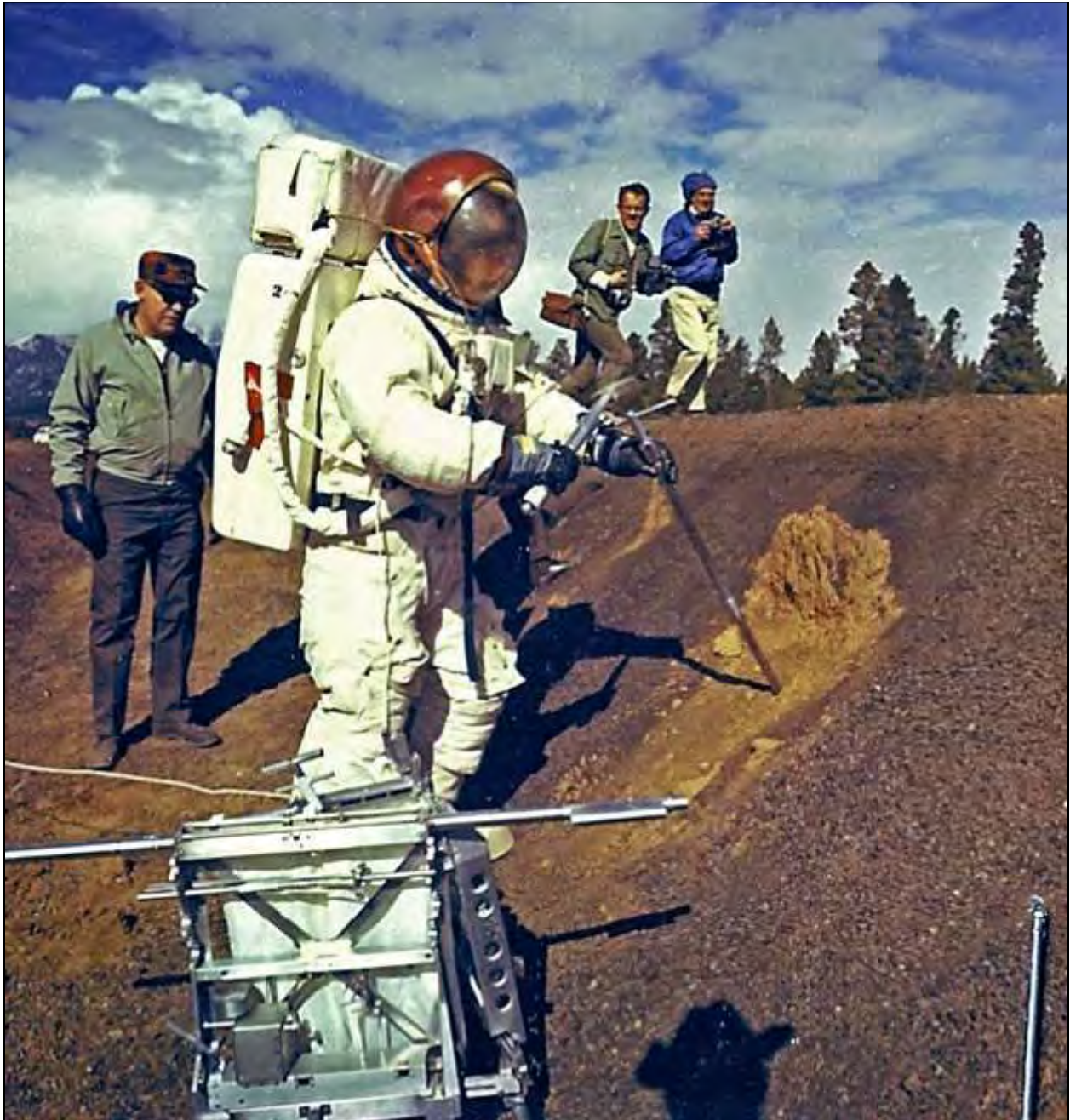
Fig. 72. Suited test subject Tim Hait drives a core sample tube into the rim of a crater at Cinder Lake Crater Field One. Note the prototype tool carrier in the foreground. Astronauts used similar tool carriers during Apollo 12-14 moonwalks. (Image from Schaber, open-file report, 2005. USGS photo P564, F36819c.)
