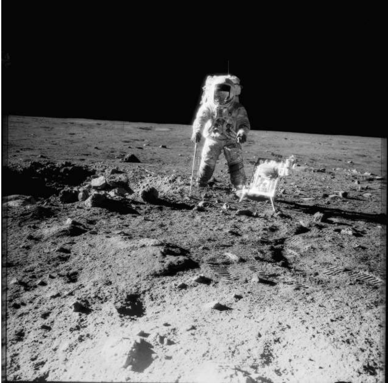
Fig. 74. Apollo 12 astronaut using lunar hand tools and a carrier similar to the one tested at Crater Field One. (November 19-20, 1969, NASA photo AS12-49-7318.) Image available from: https://spaceflight.nasa.gov/gallery/images/apollo/apollo12/html/as12-49-7318.html
