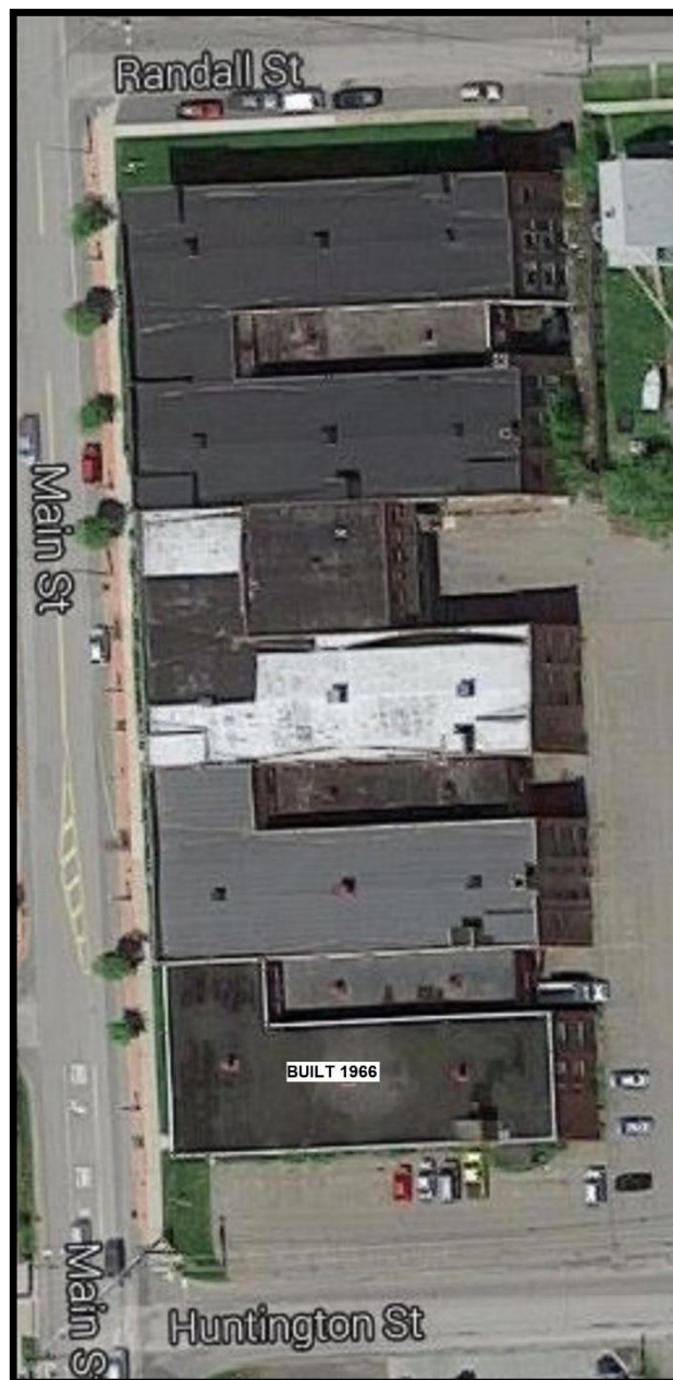
Figure 2. 2015 Google Maps Aerial View, showing complete factory with infill between Sections 1/2; 3/4, and 4/5. The loading dock between Sections 2 and 3 has also been expanded.
