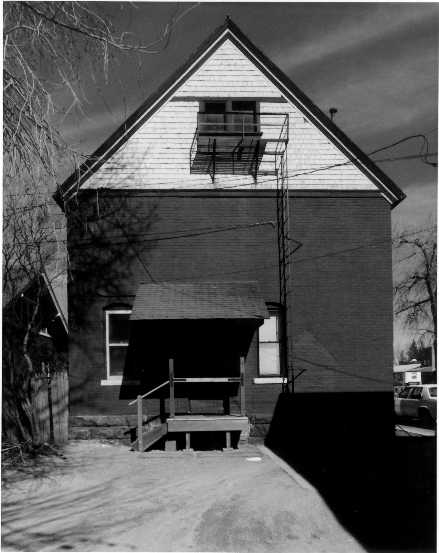
Rear elevation. Old enclosed porch replaced with open railed stoop. Original roof is retained. Shingle siding on upper gable. Continuous lintel on third floor windows. Detail of foundation stone.
