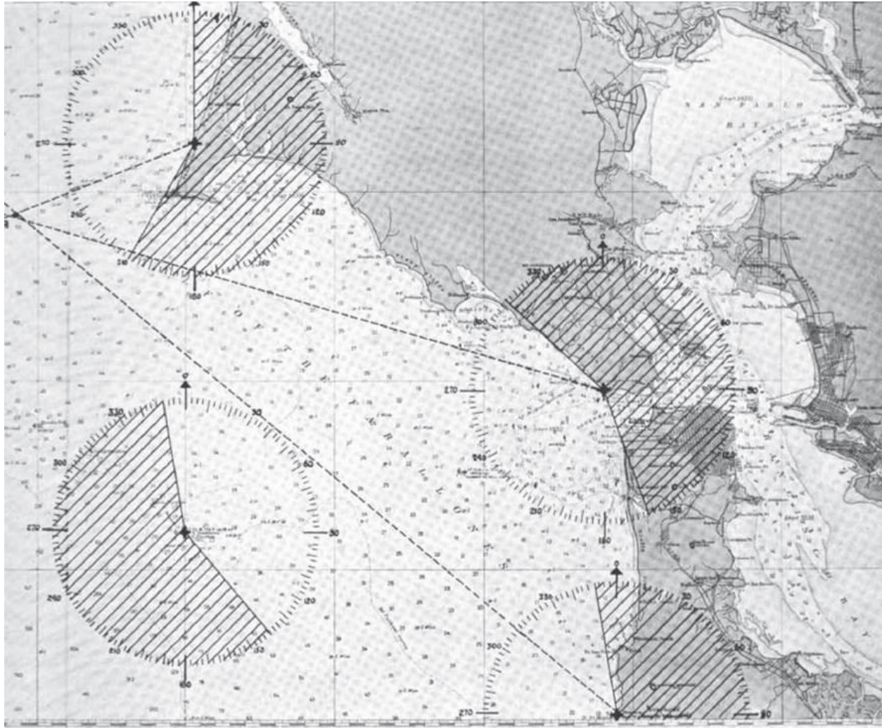
Figure 13. Map showing the blind angles of the four radio compass stations of the San Francisco Bay Entrance Group, 1920. The stations on the coastline from north to south include the Point Reyes, Bird Island, and Point Montara radio compass stations. The radio compass station on Southeast Farallon Island is located in the lower left corner. ( Pacific Marin Review )
